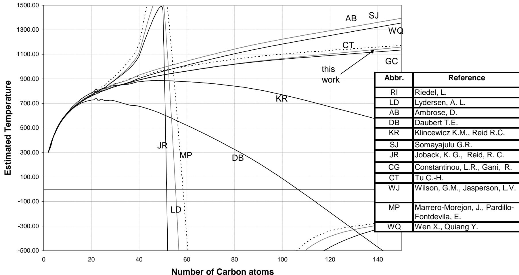
Estimated critical temperature for n-alkanes as function of the number of carbon atoms from different group contribution methods (AB and SJ overlap).
