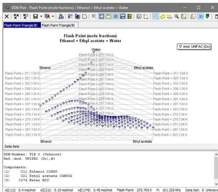
Figure 8: Flashpoint diagram of a ternary mixture.
