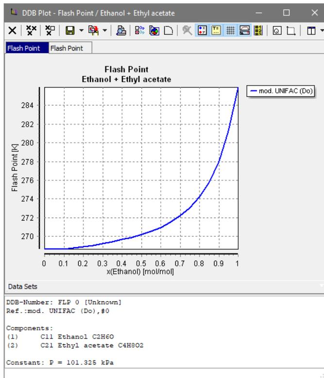
Figure 9: Flashpoint diagram of a binary mixture.
