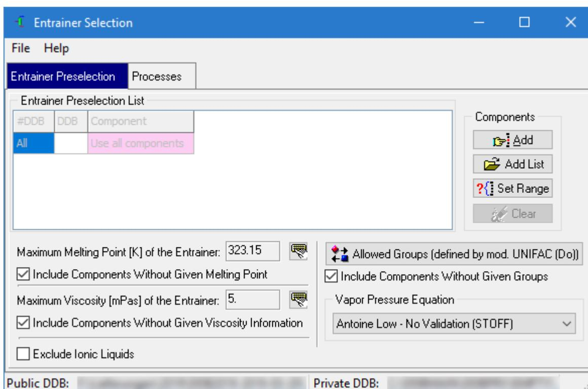
The dialog offers the possibility to specify the component range. This is useful, if the azeotropic data are calculated with a thermodynamic model. Instead of calculating the homogeneous and heterogeneous points for many thousands of components, it can be chosen between a component range (e. g. Components 1 – 500) and a component list. The component list is a “\*.stl” file, which can be easily edited e. g. in ComponentSelection.
