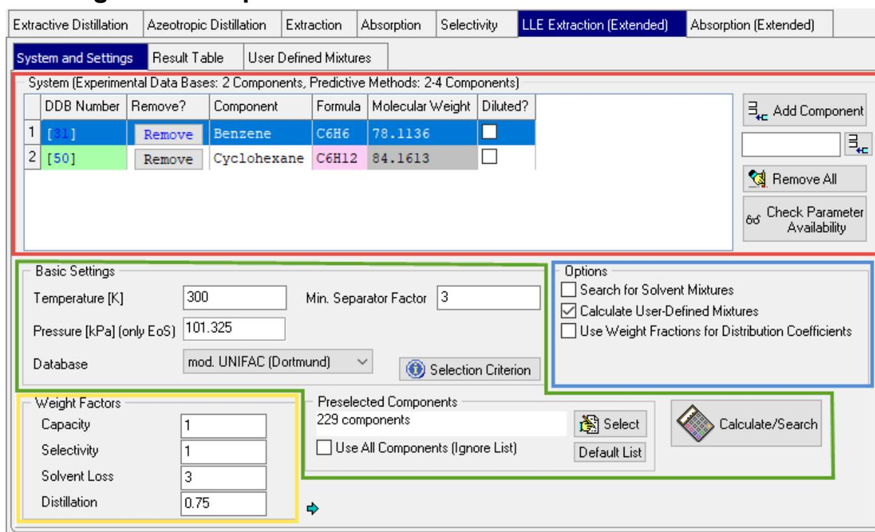
Figure 3: Main dialog of the liquid-liquid extraction (extended) program part
