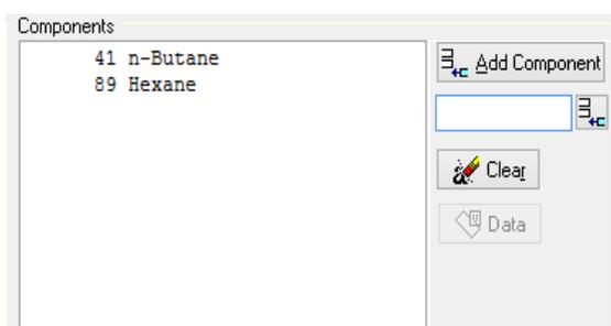
After selecting at least two components (see Figure 3) the VLE and HPV data banks are searched for the binary data sets.
