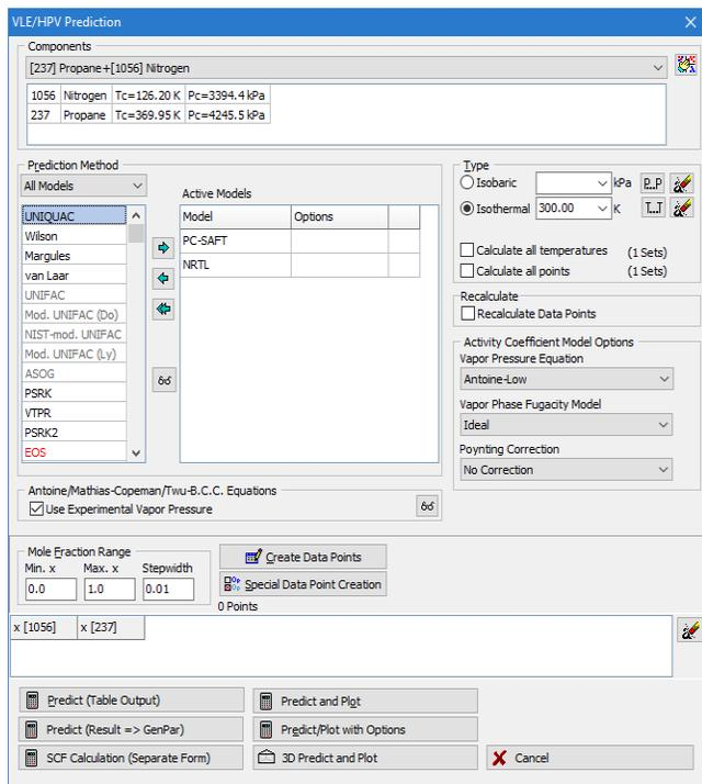
The dialog allows the selection of the predictive methods and the specification of the conditions.
